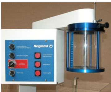
Dosing unit and control panel
