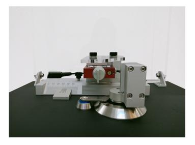
For the determination of bending resistance and stiffness of paper and paperboard
