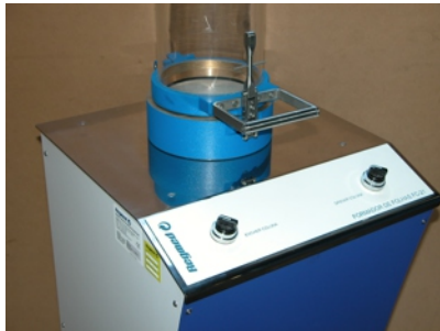
Pneumatic controls for filling, mixing and draining
