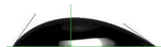
Sample Drop on Tilting Base showing Advancing Angle (left side) and Receding Angle (right side)
