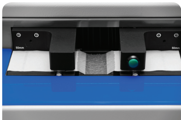
Figure: Water bath for wet tensile measurements. Measurements for up to 50 mm wide stripes possible. The tensile test ranges from 50 mm to 180 mm distance between the clamps.
