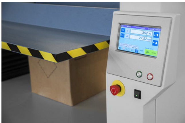
Figure: Touch screen controlled operation and display of results, stats and graphs.
