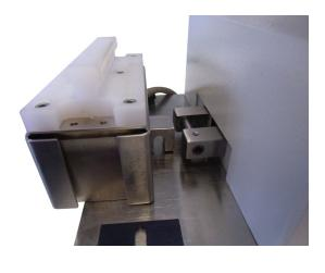
To determine the ink abrasion resistance and dirtiness characteristics on different supports (paper, cardboard, ceramic, etc.)
