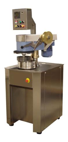
For use in the laboratory for beating of chemical pulps under standardized conditions and also for the desfibration of semi-digested raw material fibers.
