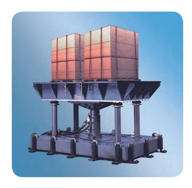
The Model 10000 Vibration Test System is designed for testing large, heavy payloads. The actuator force and large table options make the Model 10000 the ideal vibration system for testing unit loads and large crated products. The Model 10000 performs testing per ASTM, ISTA, ISO and other common industry test specifications. The system will also run test profiles created from SAVER™ environmental data.
