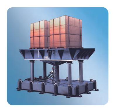
The Model 65000 Vibration Test System is the largest force system in our line of vibration equipment. Designed for testing very large payloads, the Model 65000 can be outfitted with the large test platforms that we have to offer, measuring up to 10 ft. (3 m) in length.
