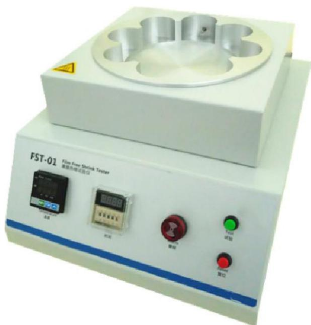
The Film Free Shrink Tester determines the degree of unrestrained linear thermal shrinkage at given temperatures of plastic film and sheeting in fluid medium.
