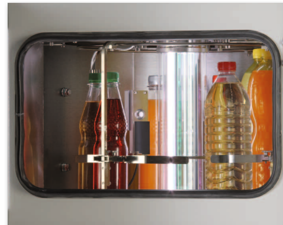
Air-cooled rotating rack test chamber including xenon lamp, optical filter lantern, and light monitor
