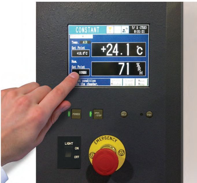
Access to the SCP-220 programmer is on the new console mounted on the left side of the door.
