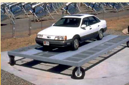
Sun-tracking carousel for automotive temperature measurement programs
