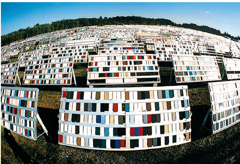
Racks in the direct weathering test field - South Florida
