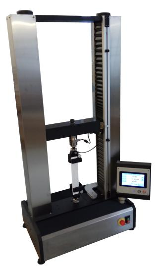
For tensile or compression tests on different materials
