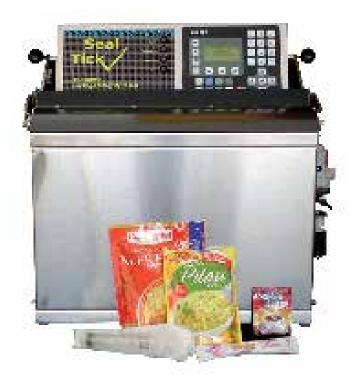
The package integrity tester (P.I.T.) uses a vacuum method to measure the gasleaking from a wide range of flexible pack types and sizes. Items are placed manually into the unit, and the handle is closed to initiate the test sequence. Results are displayed as a Pass or Fail, along with a quantitative measure of the leakage rate.
