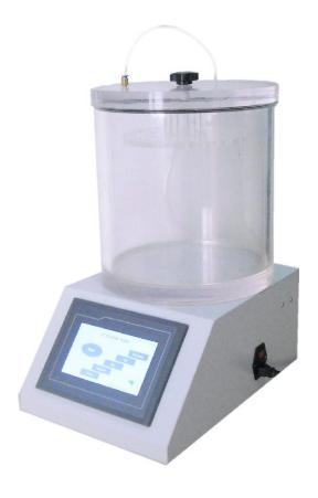
The RYCOLAB Leak Tester is used for the airproof checking of packages, containers, bags, pipes that are used in food, beverage, pharmaceutical, daily chemical, cosmetic and electronic industries, etc. It complies with ASTM D3078 and GB/T 15171 standards and could be modified to ASTM F 2054 Bubble Test.
